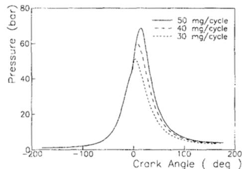
**Fig. 7** The effect of fuel injection amount on the cylinder pressure at engine speed 1200 rpm
