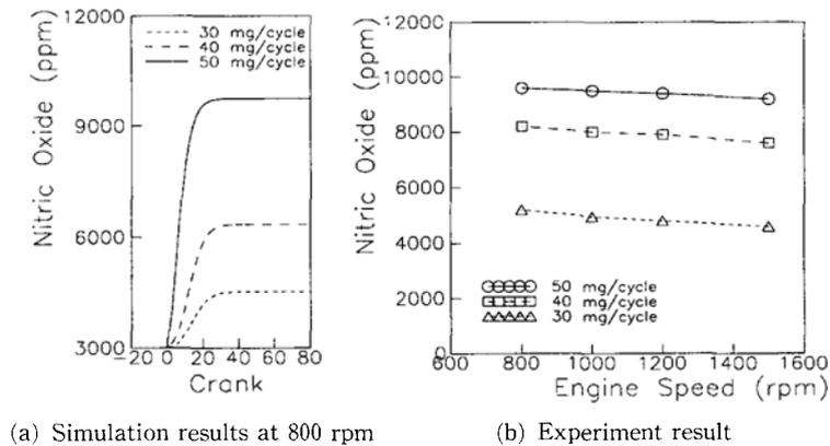
**Fig. 9** The effect of fuel injection on the nitric oxide emission
