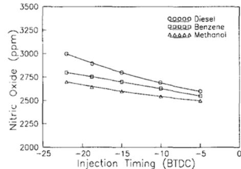
**Fig. 10** The effect of fuel injection timing on the nitric oxide at different fuel properties
