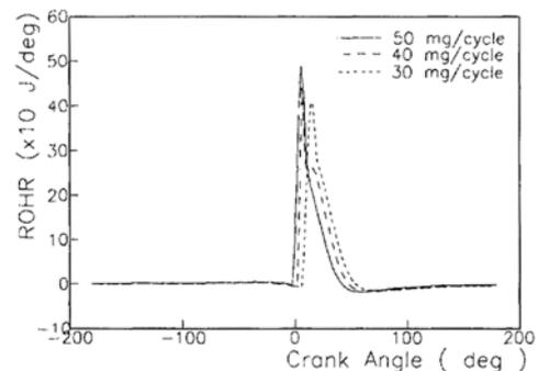
**Fig. 8** The effect of fuel injection amount on the rate of heat release at engine speed 1200 rpm
