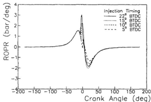
**Fig. 6** The effect of injection timing on the rate of pressure rise
