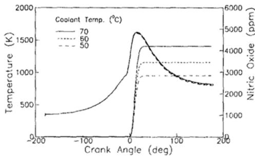
**Fig. 11** The effect of cooling temperature on the nitric oxide
