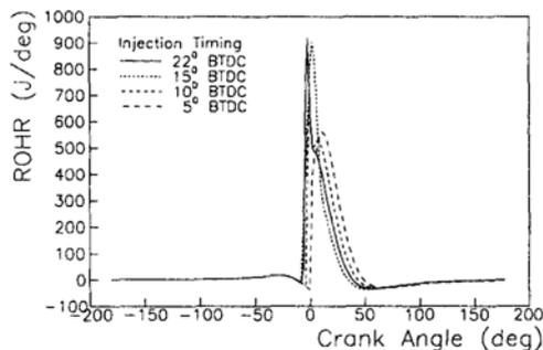
**Fig. 5** The effect of injection timing on the rate of heat release
