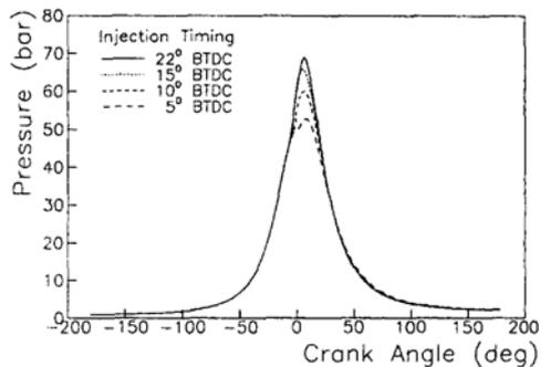
**Fig. 4** The effect of injection timing on the cylinder pressure
