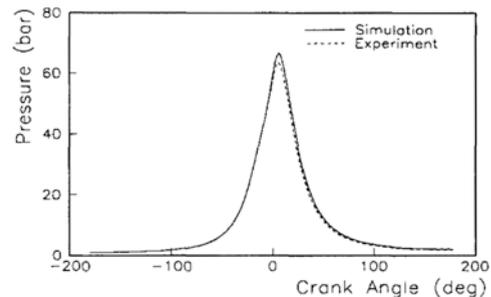
**Fig. 2** Comparison of simulation and experiment results for cylinder pressure
