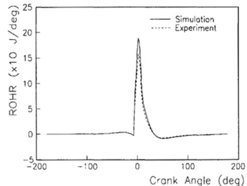
**Fig. 3** Comparison of simulation and experiment results for rate of heat release
